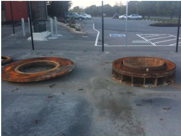
Original base & turntable, Biotower No. 2
